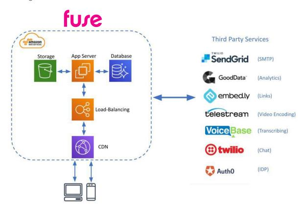
Fuse utilises many of the core AWS services such as EC2 (Application Server), S3 (Content Store), RDS Aurora (Database), ELB (Load-balancing), Route53 (DNS).
